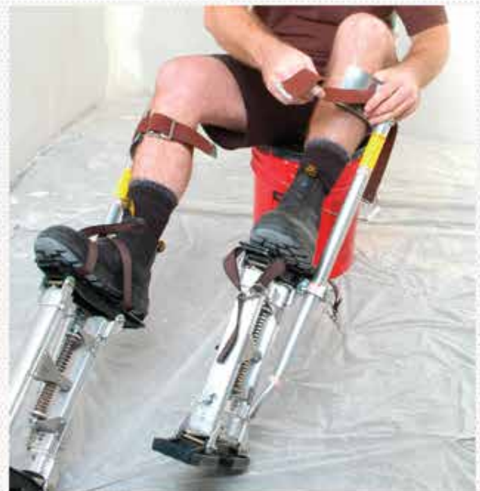
■ Upper foam rubber leg pads are comfortable on the calf
